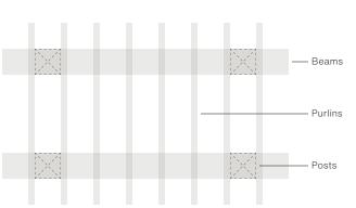
Beams and purlins extend 16" past post positions on all pergolas except Vineyard. Vineyard beams and purlins extend 1.5" past post. Pergolas 22' and above will have 6 posts. Length must be equal or greater than the width.
