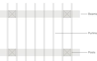
Beams and purlins extend 16" past post positions. Pergolas 22' and above will have 6 posts. Length must be equal or greater than the width. \*18' width is not available with deluxe shade.
