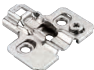
600.OP71.05 COLD ROLLED STEEL, NICKEL PLATED 600.OP73.05 COLD ROLLED STEEL, NICKEL PLATED ■ PREASSEMBLED WITH 6.3MM X 15MM EURO SYSTEM SCREWS ■ HEIGHT ADJUSTMENT: +/- 2MM
