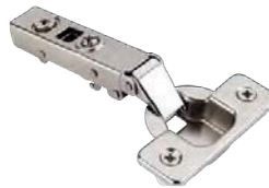
700.0181.25 FULL OVERLAY 0MM CRANK PRESS-IN 8MM DOWELS CAM ADJUST
