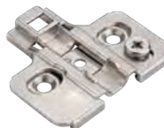
600.OP72.05 ZINC DIE CAST, NICKEL PLATED 600.OP74.05 ZINC DIE CAST, NICKEL PLATED ■ PREASSEMBLED WITH 6.3MM X 15MM EURO SYSTEM SCREWS ■ HEIGHT ADJUSTMENT: +/- 2MM
