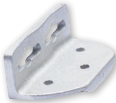
B20-4 CAST ALUMINUM 4 3/8" H X 2 1/8" W ■ NEEDS SAW CUT IN RAIL ■ 3 #8 SCREWS ■ 2 LAGS ON POST ■ LEFT AND RIGHT UNIVERSAL ■ SCREWS, LAGS, AND RUBBER HEAD COVER INCLUDED
